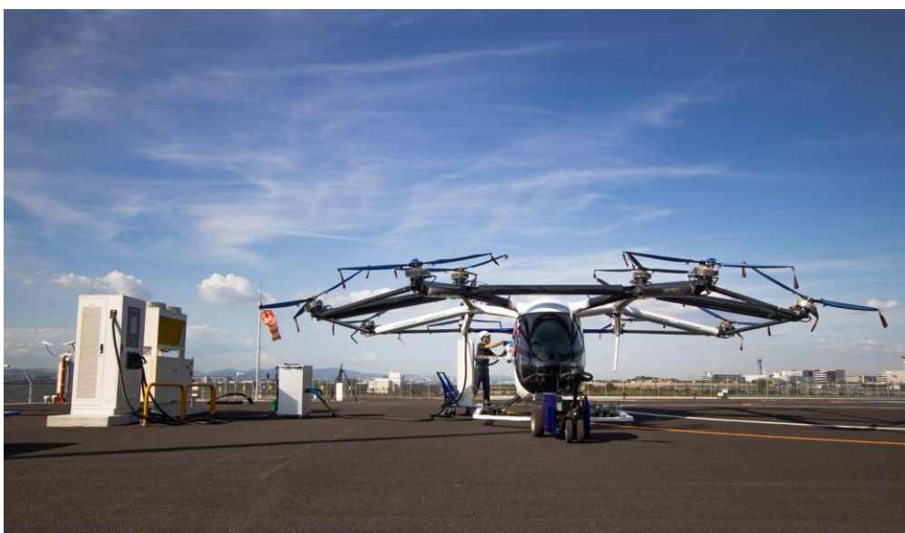
The SKYDRIVE, seen here getting charged, is an all-electric aircraft with a batteries rather than aircraft engines
